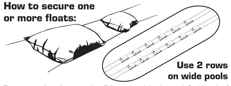
Floats are joined together using a 3mm Poly rope (eg; clothes line rope). Cut 2 lengths of rope (per row of floats) 2 metres longer than the length of the pool. Details overleaf.
