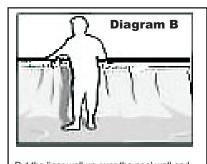
Put the liner wall up over the pool wall and hold in place with the plastic coping strips. Adjust the overlap to remove all wrinkles.
